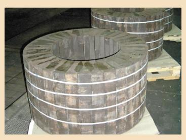
That is why especially responsible areas of refractory linings are fully executed at the manufacturer's premises more and more frequently, which enables to ensure required conditions of the technological process and achievement of expected operational parameters.
